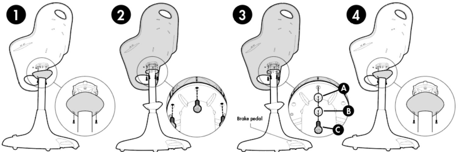
**1** Remove the (2) M4 bolts that attach the seat base. Do not discard these bolts. Remove the seat base cover.
